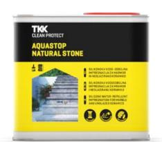
Aquastop Natural Stone is a colourless liquid based on silane-siloxanes and special additives in organic solvent for the final protection of porous (absorbent) inorganic materials against water and moisture. Because of its high absorbency, it penetrates deep into the pores of the material and, after the solvent evaporates, forms an invisible impregnation of the surface with no film formation.
