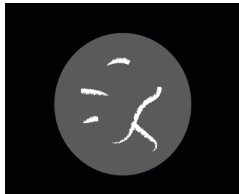
Noticeably white stripes – bad mixing quality
